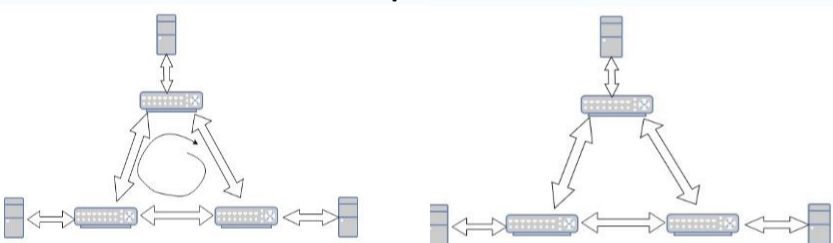
Broadcast streams in a network having a loop structure logically disconnect to avoid loop using STP.
